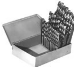
11 PIECE HD 135° SPLIT POINT JOBBER LENGTH GOLD M42 COBALT 1.0-6.0mm X 0.5mm Code: 754715
